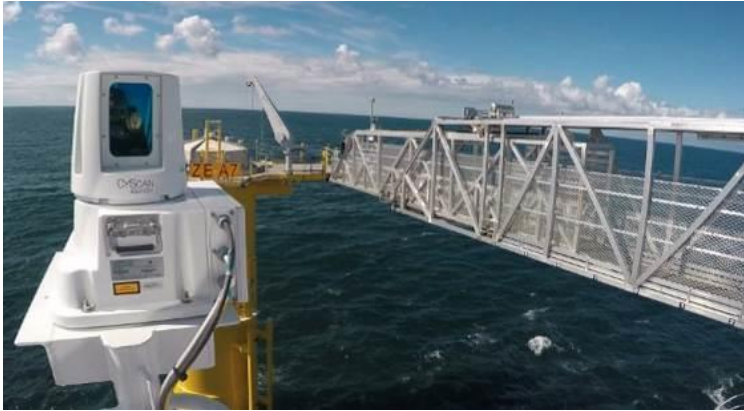
Figure 6. CyScan Sensor on the Windea La Cour. The CyScan is slightly higher than the Motion compensated gangway, which is 12-13m higher than the RangeGuard sensors.
