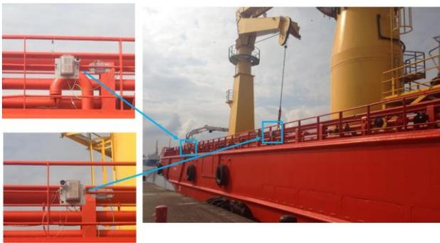
Figure 3. Locations of RangeGuard Sensors and video cameras mounted on custom brackets.
