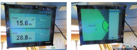
Figure 4. Display on the bridge. Different views are available on the user interface. Left: Range and speed information from the two sensors, Right: Birds eye view showing the vessel and sensor beam patterns.
